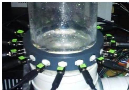
Figure 9. Ultrasonic transceiver arrangement with sensor jig
