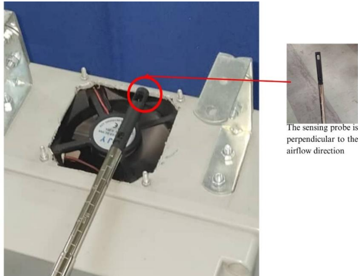
Figure 13. The measuring of the exhaust fan airflow using anemometer
